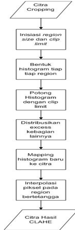
Gambar 7. Diagram Alir Proses CLAHE
